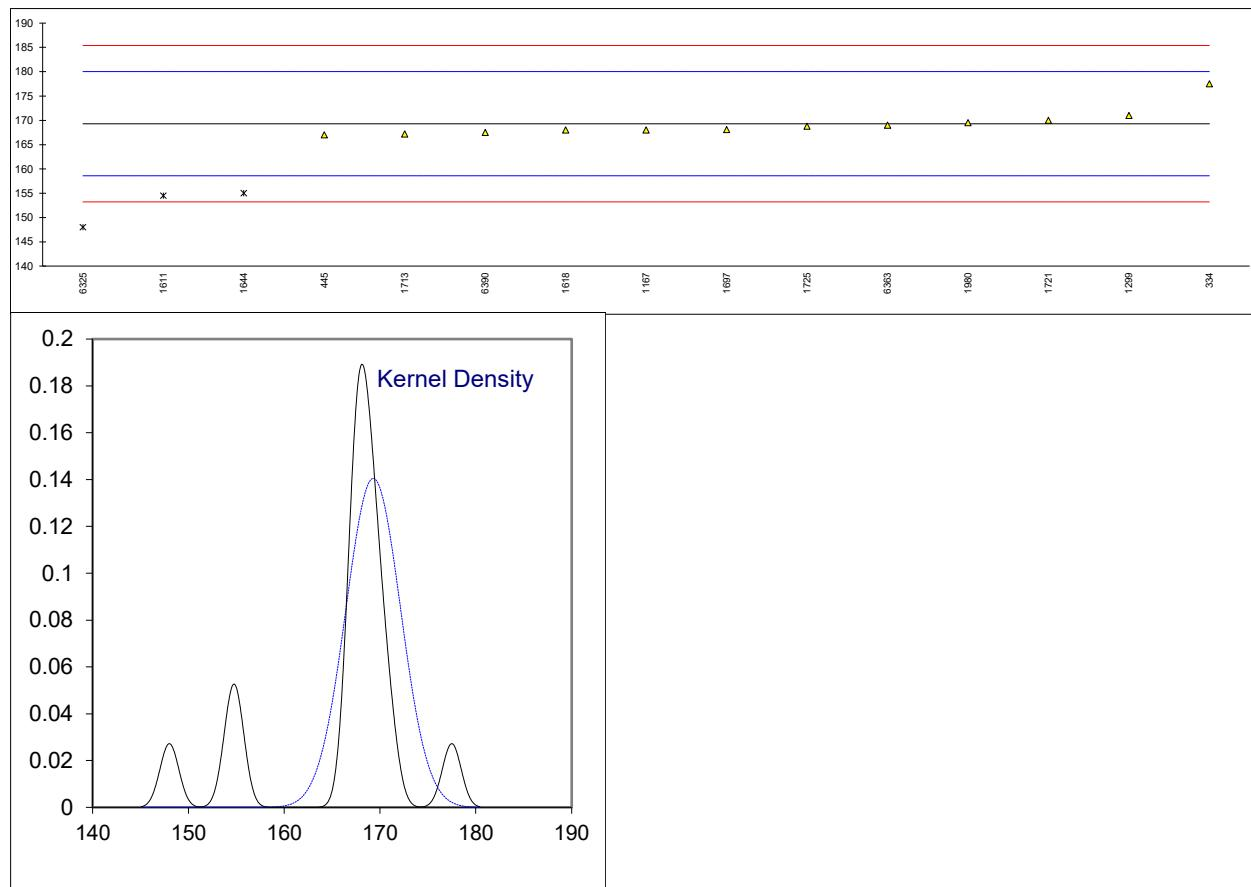
Determination of Iodine Value on sample #21055; results in g I<sub>2</sub>/100g
